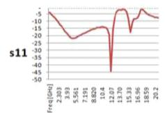
Fig. 3: Return loss without using stacked DRA
