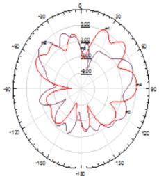
Fig. 7: Radiation Pattern using 20V DC bias
